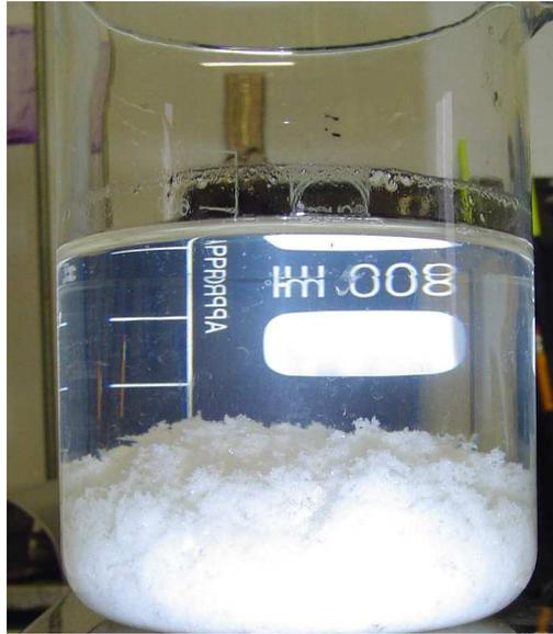
The product **HYCOR EBCL** reacts simultaneously with metals, suspended solids and oil and grease to form large, dense flock that settles efficiently, resulting in improved performance of the clarifier, shorter filter press cycles and drier filter press cakes. The treatment proved very economical and versatile, and the product is easy to work with and safe to handle. The new treatment produces effluents that meet or exceed discharge standards and generates non-hazardous waste
